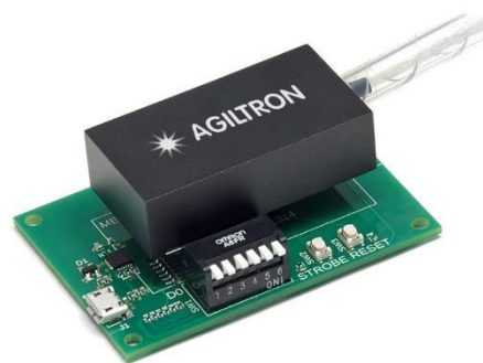
■ Mounted on USB/RS232/TTL PCB with Power Supply
